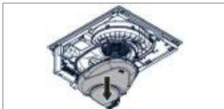
Fig. 11.28 Removing the bottom of the suction chamber
